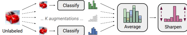
Figure 2. (Source: Berthelot et al. [2]) Diagram of the label guessing process proposed in original MixMatch . They applied stochastic data augmentation to each unlabeled image K times, and each augmented image was fed through the classifier. Then, the average of these K predictions was "sharpened" by adjusting the distribution's temperature T .
